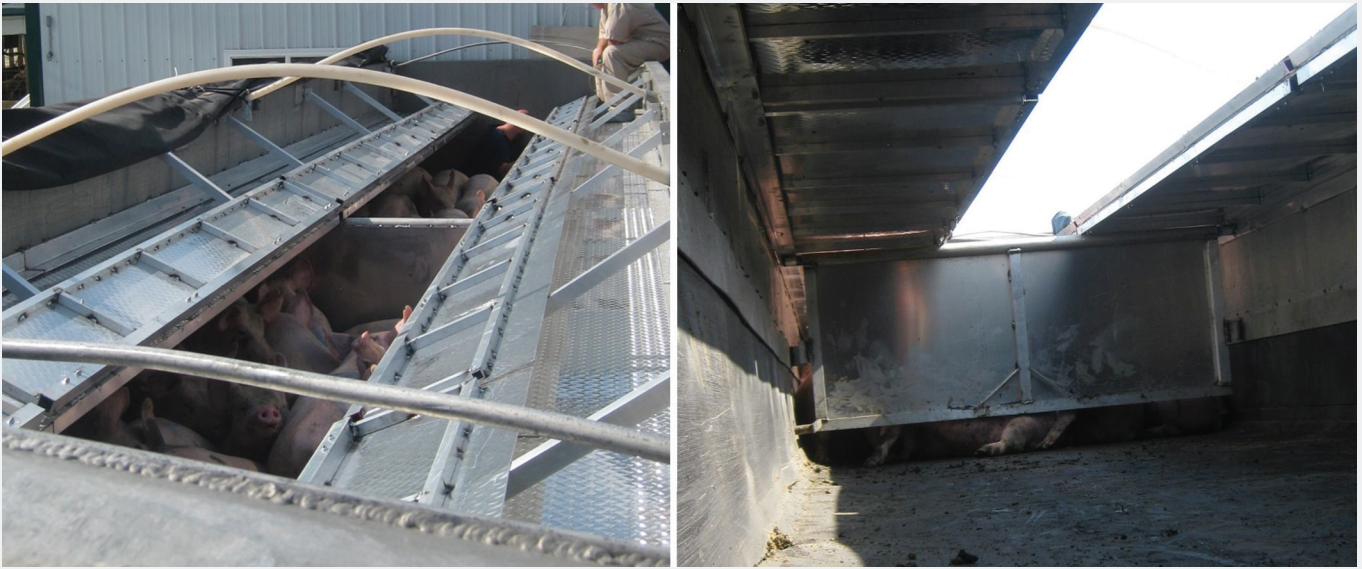
Figure 3: Top hinged swing gate installed at the halfway point of the trailer. The swing gate can be lowered after filling the front half of the trailer to allow greater ease in loading pigs in the back half.
