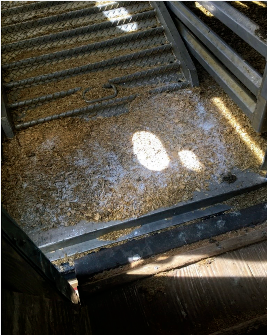
Figure 4: The mixture of fluorescent powder (Glo Germ), wood chips and obstetrics gel placed just inside the roll up door of the livestock trailer. The fluorescent powder appears white in sunlight and fluoresces when the primary light source is long-wave ultraviolet.
