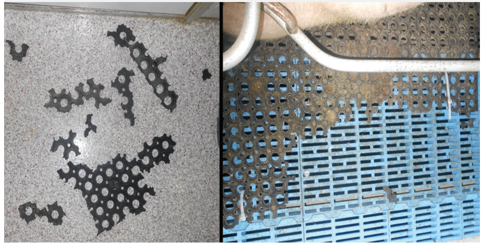
Figure 1: A 99 × 150 × 1.4-cm heavy-duty rubber mat damaged by the sow during the day prior to farrowing. Note the different sizes of fragments (7.5 to 25 cm) as well as the damaged area in the rubber mat on the right (approximately 25 × 75 cm).
